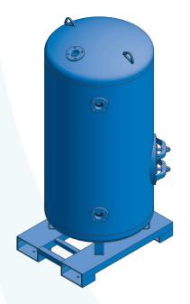
Jumbo-Type, Portable Exchange Deionziation Tanks (PEDI) are used for larger, high purity water treatment applications where the convenience for using an off-site resin regeneration service is desired. Suitable for a variety of system configurations including Separate-Bed DI, Mixed-Bed DI, Specific Ion Resins, and Filtration Media.
